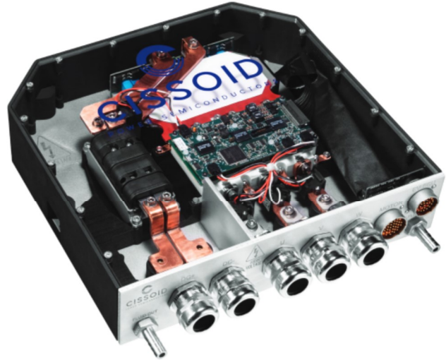
This Cissoid/Silicon Mobility's modular inverter reference design drives 350 kW/850 V motors (Image courtesy of Cissoid)
