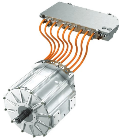
Dana’s HD motor/inverter system has a nine-phase HV inverter with variable switching frequency, Reflex technology gate drivers and an EMI filter (Image courtesy of Dana TM4)
